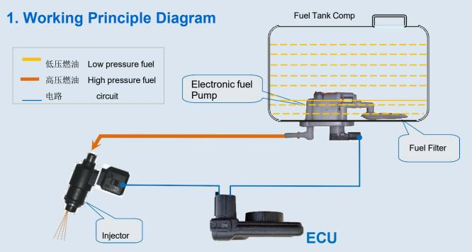
The fuel pump is controlled by the ECU, there is a one-way valve at the oil outlet of the fuel pump. When the engine is not working, the fuel in the fuel pipe will not back to the fuel tank. This ensures that the fuel pump supply pressure is 300KPa when the engine is started again.
