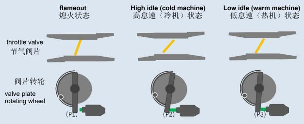
The stepping motor is controlled by the ECU. It's a actuator to achieve idle speed at a set target value.
